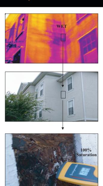
Using thermal imaging, we can evaluate the condition of exterior cladding systems by mapping areas of moisture entrapment and delamination due to environmental stress.
