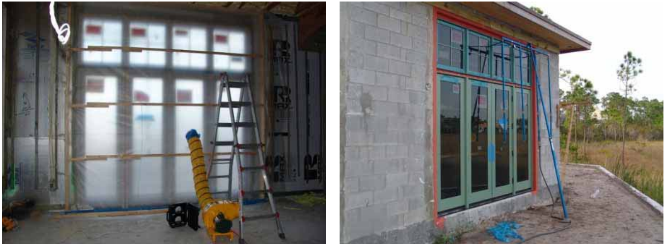
Figure 2. Photo of chamber system, negative air fan, pressure monitor, and calibrated spray rack system.
